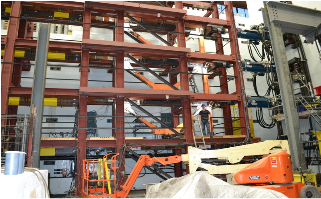
Figure 2.11: large-scale steel structure with viscous dampers (NEES project 1018, Dong et al., 2014 ).
