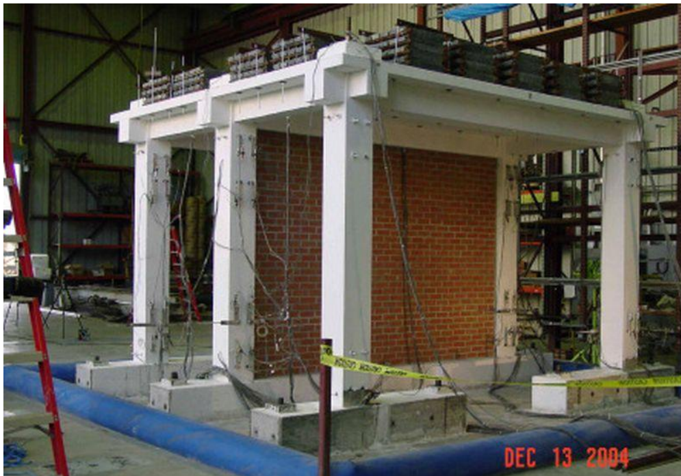
Figure 2.3: Experimental substructure conformed by RC frame and URM infill in the middle (NEES project 135, https://nees.org/warehouse/experiment/205/project/135 )
