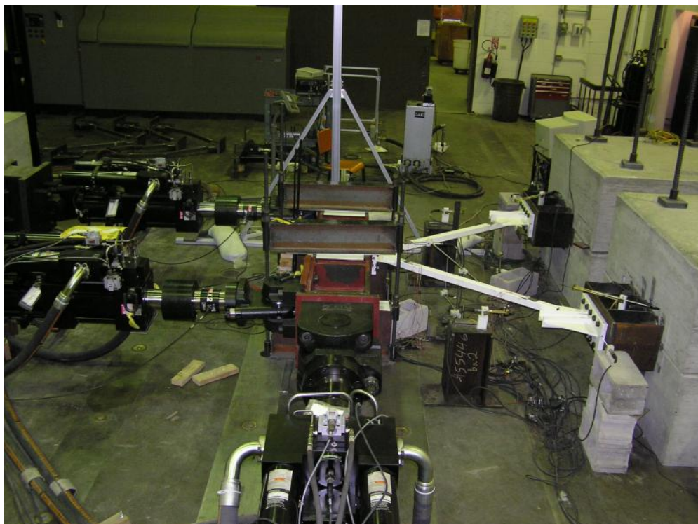
Figure 2.7: Experimental substructure of the suspended-zipper braced frame (NEES project 24, https://nees.org/warehouse/experiment/110/project/24 ).
