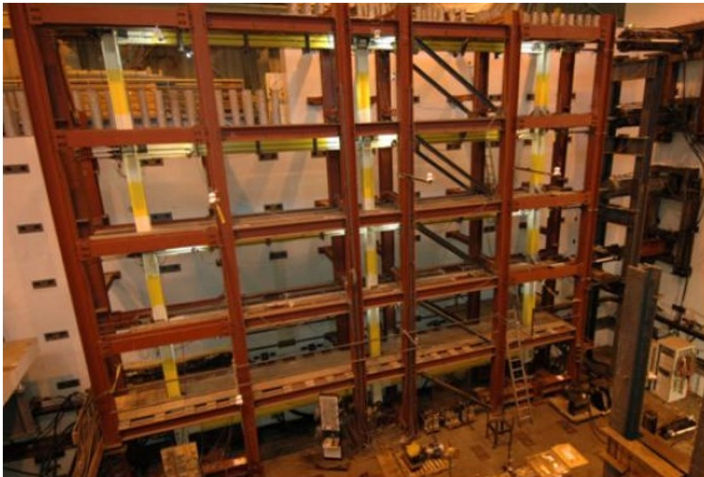
Figure 2.8: SC-MRF 4-story test frame with lateral loading as experimental substructure (NEES project 77, https://nees.org/warehouse/experiment/1151/project/77 ).
